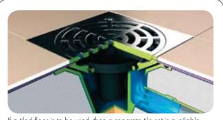
If a tiled floor is to be used, then a separate tile set is available. This is then fixed directly over the outlet mouth and the grating is removable to allow full access to the trap unit.
